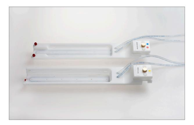
The rat and mouse bed bases are used in combination with bed tips to hold the animal in place during imaging, as well as to deliver gas anesthesia and heat the animal during scanning.
