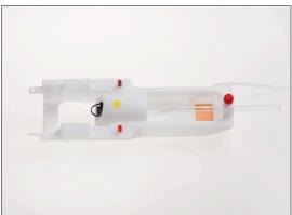
The rat brain phased array is used for receiving the MR signal from the rat brain. It should be used in combination with the 72 mm transmit coil (see page 7).
