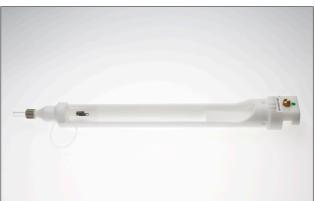
The 60 mm ID quadrature coil is used for exciting and receiving the MR signal from the rat body, providing the rat fits easily into the coil (in general, the rat should not weigh much more than 300 g as then the signal-to-noise ratio achieved by the coil is reduced).
